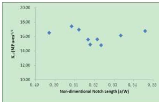
**Fig. 5.** The relationship between  $K_{IC}$  and  $(a/W)$
