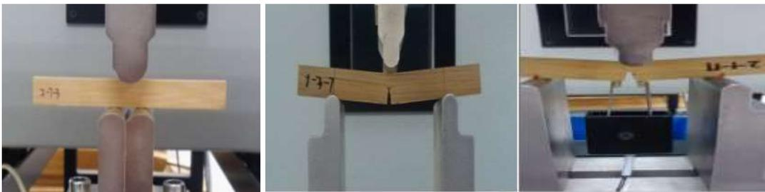
**Fig. 2.** SENB testing according to ISO 13586-2000 and ASTM E399-09
