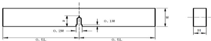
Fig. 1. Schematic diagram of the sample dimensions with the notch
