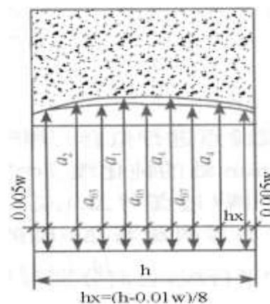
**Fig. 3.** Measurement of pre-crack length  $a$
