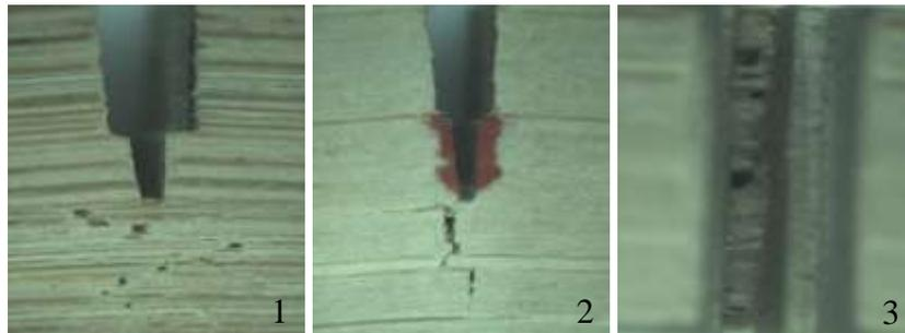
Fig. 6. Failure mode of bamboo specimen
