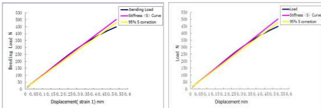
Fig. 4. Stiffness method to determine the initial crack load
